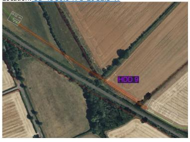
**HDD 8: Example for Railway crossing (33kV cable)**
